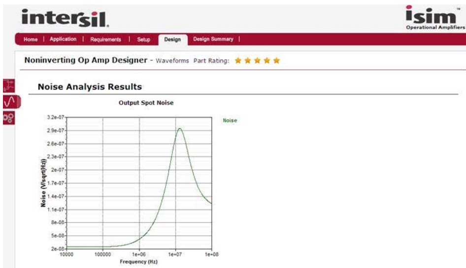
FIGURE 13. SPOT OUTPUT NOISE WITH R_f = 5.1k\Omega REDESIGN
